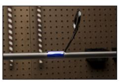
**PRO TIP:** Never apply heat directly to the epoxy as too much will create more bubbles or harm components.
