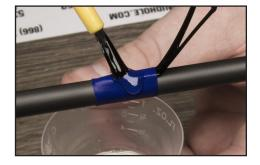
**PRO TIP:** Do not glob on epoxy, apply evenly to thread and touch up bare thread spots as you go.
