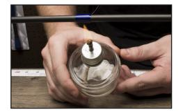
**PRO TIP:** Never apply heat directly to the epoxy, as too much will create more bubbles or harm components.
