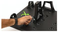
**2.** Start with the uprights(C). These connect the base plate(B) to the top plates(A). When installing the uprights, your nylon nuts and washers go on top, as there is a recessed hole to fit the cap head crew on the bottom of the base plate.
