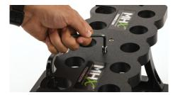
**3.** Once your uprights are installed, you will see there are two threaded inserts on the top of the uprights. Line up the screw holes on the top plate to the threaded inserts on the uprights and be sure the removable wing braces line up with the bent butt gimbal pins at each of the four corners of the base plate. Now secure the top plates to the uprights with the cap head.
