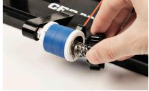
5. With all parts now fully assembled, choose your favorite thread color. To install, unscrew the knob from the threaded rod on the carriage. The following assembly is recommended - from the nut moving outward: Large OD Washer, Spool of Thread, Large OD Washer, Spring, Small OD Washer, Knob.
