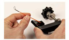
1. Install the orange Tension Rod (G). Included is a small stick of heat melt glue (H). Carefully heat one end of the glue stick until it begins to soften and dab some glue onto the end of the tension rod. Install the Tension Rod into the small hole on the front of the thread assembly, making sure the Tension Rod is fully seated and the tip top is facing up.
