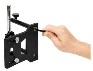
3. Rotate the Base Plate onto its edge while inserting one Upright Screw (D) into the countersunk screw holes from the underside of the Base Plate. The Upright Screw threads into the bottom of one of the Uprights (B). Loosely tighten with Assembly Tool (J). Once each side of the Uprights are attached, fully tighten each Upright Screw, alternating each screw until both are completely seated and tight.
