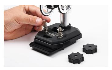
4. Slide each tension spring (E) back over each threaded bolt (D). The wide end of the spring should be facing down and resting on the Roller Stand Base. Place each washer (F) on top of each tension spring (E).
