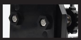
The threaded bolts rest in a slot under the baseplate. There is no need to remove the bolt. If it becomes unseated it will not allow the tension knob to fully tighten. To prevent the bolt from moving, assemble the adapter plate on a flat surface.
