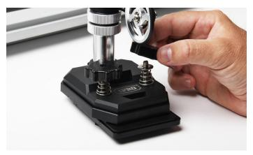
2. With the Adapter Plate resting on a flat surface, unscrew each round tension knob (G) and remove. Remove each washer (F) and tension spring (E) from the threaded bolt. Keep these close at hand as you will use them during reassembly.
