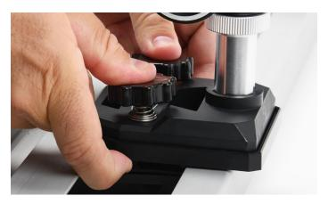
6. Start at the open end of your C-Channel track System. Using your thumbs, depress the tension springs by pushing on the tops of the tension knobs. This will allow the base plate to separate from the adapter plate providing room to slide onto the track. Once you release the tension springs the base plate and rubber gasket will make contact with the underside of the C-Channel track holding it firmly in place.
