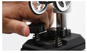
5. Add each tension knob (G) to each threaded bolt (D). Give them a few full revolutions to properly seat the knob. Additional tightening will be needed once the adapter plate is on the track. You are now ready to slide the CRB PRO Roller Stand with Adapter Plate onto your C-Channel Track System.
